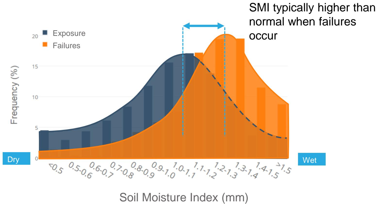
Confirmed SMI >0.9 to be an indication of conditions more prone to failure
